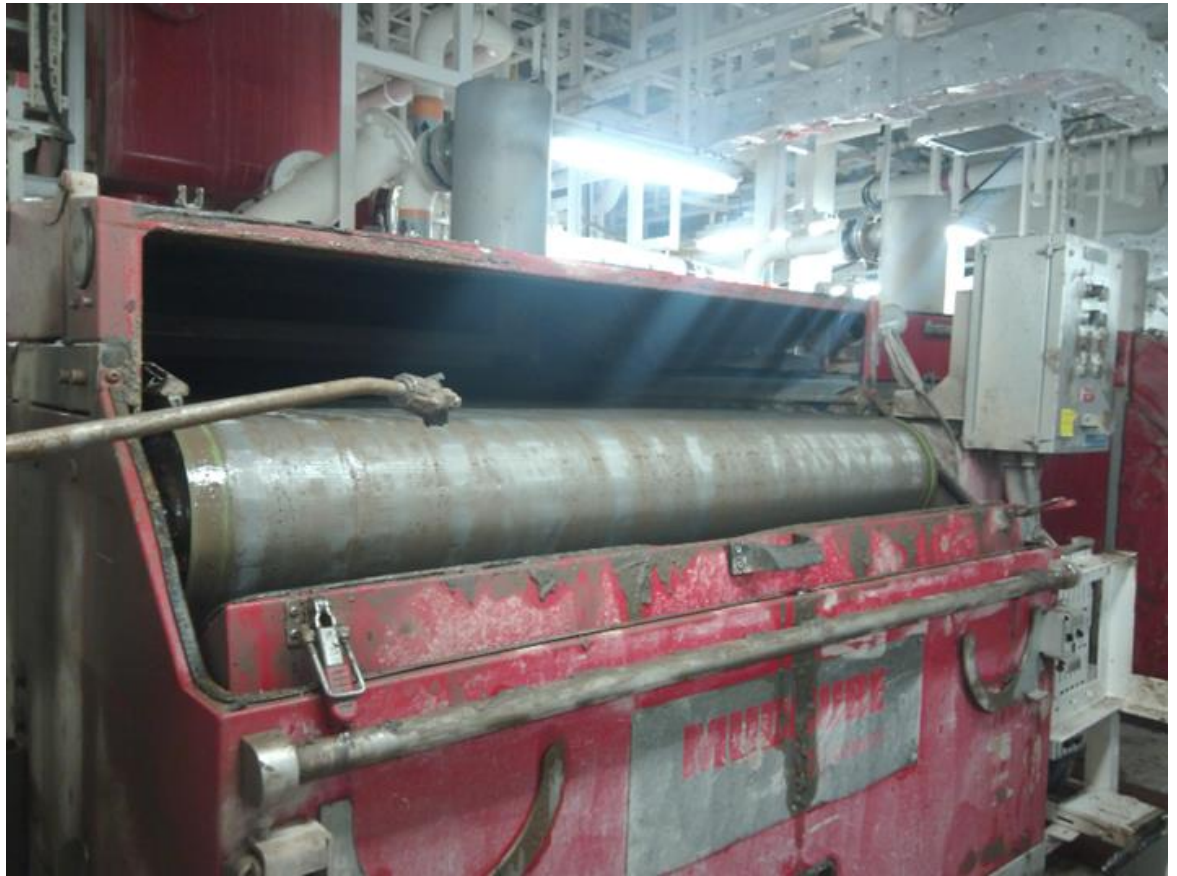
Cleaning of filterbelts (air nozzle and flushing)
